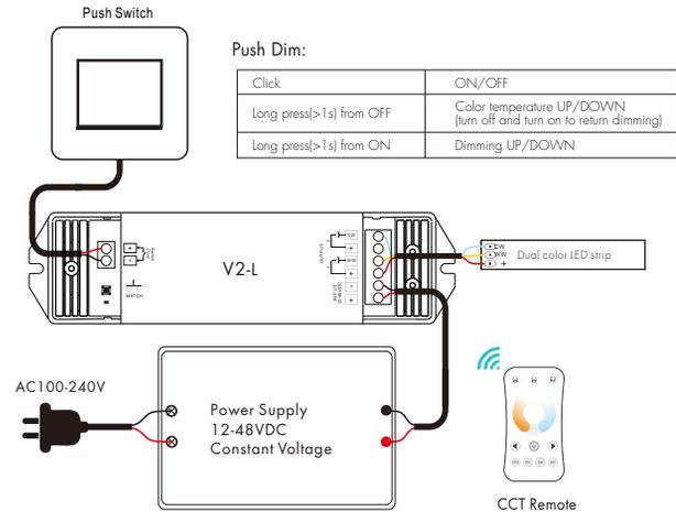
Note: Continuously switch off and on the power supply two times rapidly, It will change 3 levels color temperature (WW, NW and CW) in sequence.
